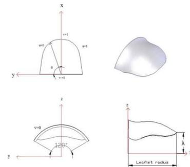
Figure 1. Coordinate system - valve leaflet.
