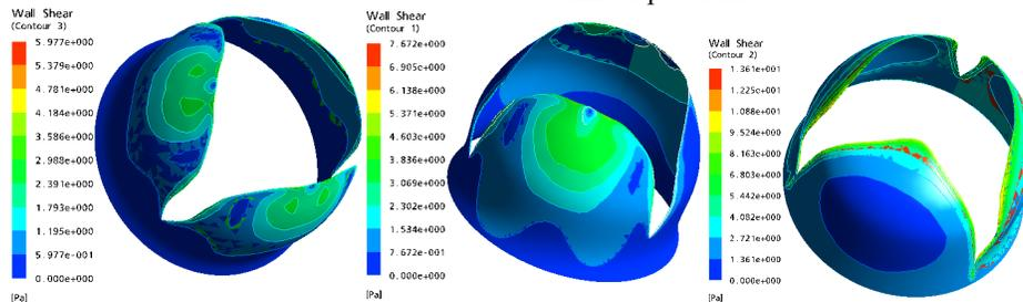
Figure 5. Shear stress distribution at case 3: (Left) Normal (Mid) Bicuspid (Right) Prolapsed
