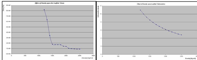
Figure 6. (Left) Density vs. Stress (Right) Density vs. deformation
