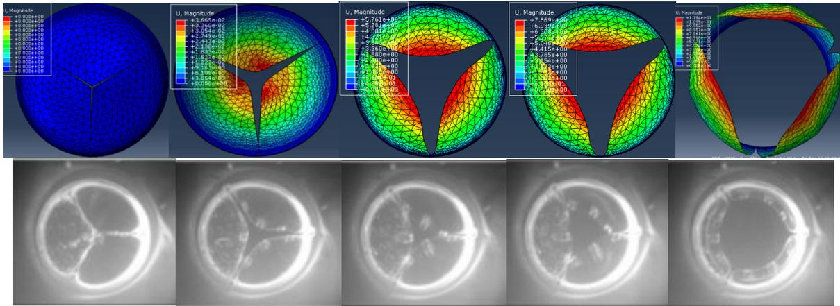
Figure 8. Heart valve leaflet deformation:(Up) Numerical (Down) Experimental [8]
