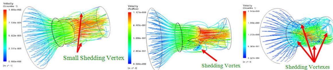
Figure 3. Flow field at case 3: (Left) Normal (Mid) Bicuspid (Right) Prolapsed
