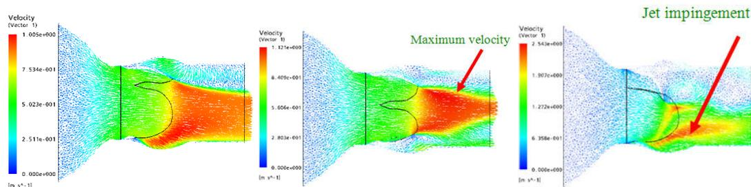
Figure 4. Velocity distribution at case 3: (Left) Normal (Mid) Bicuspid (Right) Prolapsed
